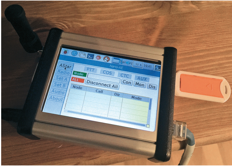
Figure 9 — The Nano-AE AllStar node. The antenna is visible on the left; on the right is a USB flash drive for backups, along with the wired ethernet connection.
