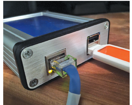
Figure 11 — The wired ethernet networking port (left) and a pair of USB 2.0 ports (right). I have a flash drive inserted into one USB port, where I can store backups.
