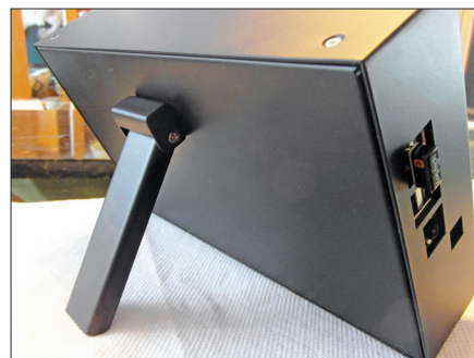
Figure 5 — There is a folding stand in the back so that the unit will be self-supporting at about 30 degrees from vertical.
